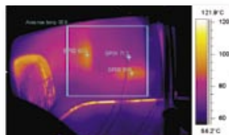
Measuring electronic components: temperature of electric pump at work
