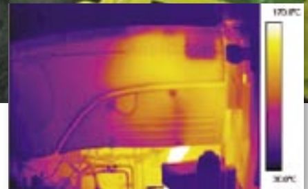
Checking hood surface temperature distribution
