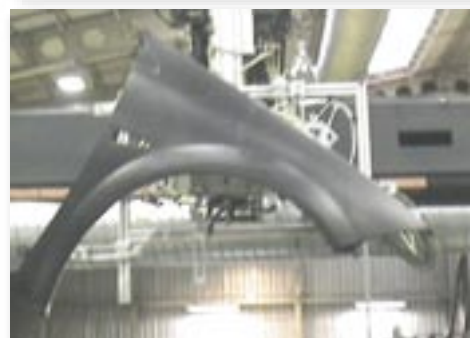
Plastic fenders: ThermoCAM S65 visualizes problem zones at the extremities
