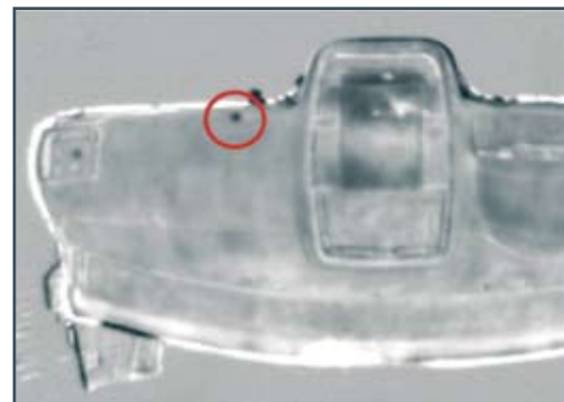
Result image showing cavities in the foam
