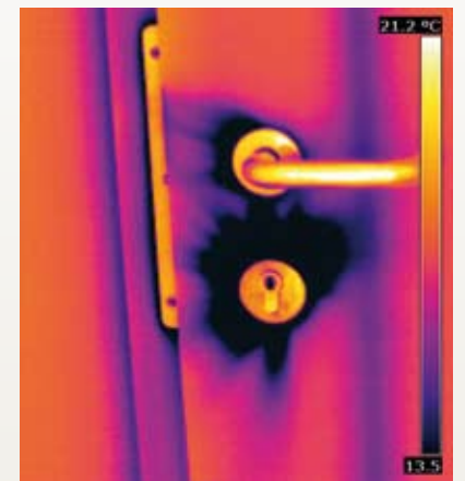
Air leaks in door with considerable temperature difference
