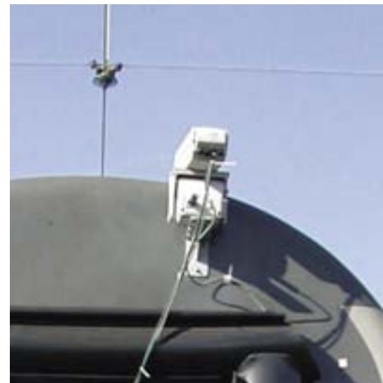
FLIR Systems ThermoVision A40 camera in housing placed on a test wagon.
